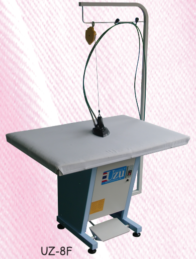
UZ-8F-VB4-A (Ironing table Built-In boilers.)
